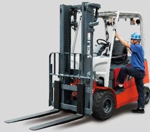
Enlarged boarding space and foot operation space offer more comfortable operation.
